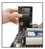
2. Locate the audio slot on the motherboard.
